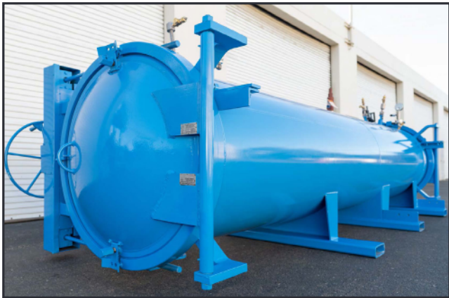
To increase chlorine held on site, while remaining within regulations, the plant will be changing to a Twin Double Ton vessel, like this one, later this year.
